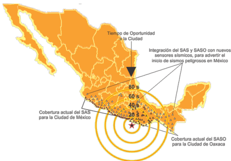
Figure 2-7 - Earthquake warning system for Mexico. The triangles correspond to the stations of the warning network and the radiating circles to the wave propagation times from the epicenter (red triangle).
